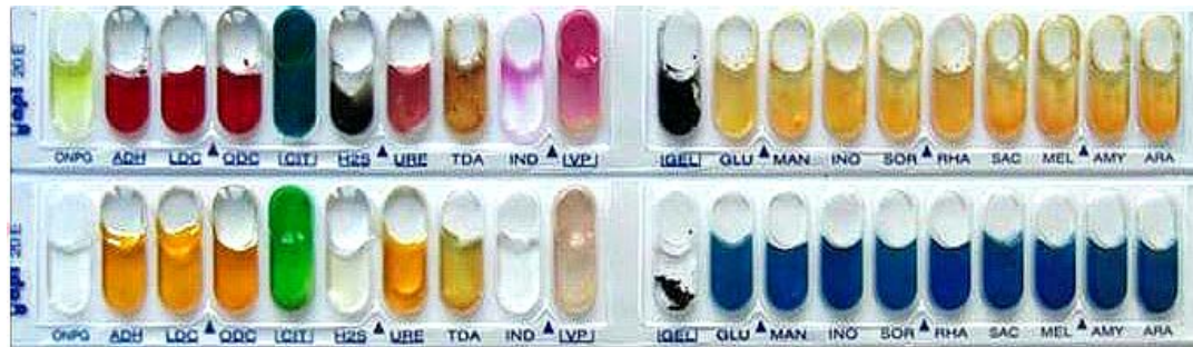
Fig. 63. API test system for enterobacteria. Upper plate – all tests positive, lower – all negative
