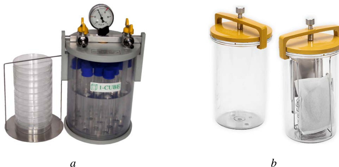
Fig. 55. Equipment for cultivating anaerobic bacteria: I-CUBE anaerostat (a) and GasPak 100 anaerostat (b)
